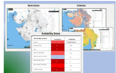
Identify sites using Analytical Hierarchy Process (AHP) by assigning weights of suitability to pre-defined criteria.
